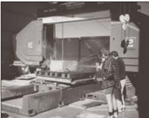
1999 "Fred Flintstone", the robot saw, was installed at the quarry thanks to a generous bequest. It has taken 4 years off the building time.
